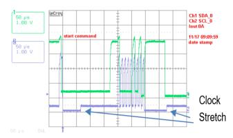
1<sup>2</sup>C Bus Lock-Up detection: The device will abort any transaction and drop off the bus if it detects the bus being held low for more than 35ms.
