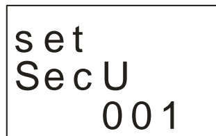
Figure 31. Secondary voltage ratio
