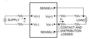
Figure 15. Circuit Configuration for remote sense.
