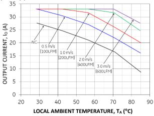
Figure 21. Output Current Derating for the Base plate QBVW033A0B-H at 48V in with 0.25" heatsink and Transverse airflow from Vin(-) to Vin(+)
