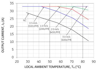
Figure 22. Output Current Derating for the Base plate QBVW033A0B-H at 48V in with 0.5" heatsink and Transverse airflow from Vin(-) to Vin(+)
