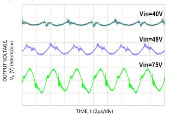
Figure 3. Typical Output Ripple and Noise,  $I_0 = I_{0.max}$ .
