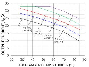
Figure 19. Output Current Derating for the Open Frame QBVW033A0B at 48V in with Transverse airflow from Vin(-) to Vin(+)
