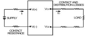
Note: All measurements are taken at the module terminals. When socketing, place Kelvin connections at module terminals to avoid measurement errors due to socket contact resistance.
