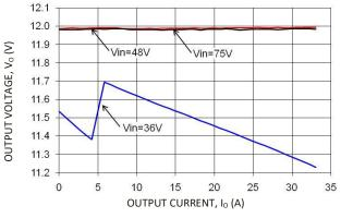
Figure 8. Typical Output Voltage Regulation vs. Output Current.
