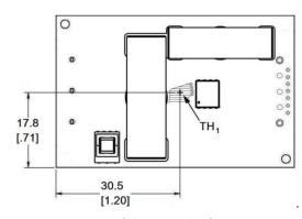
Figure 17. Location of the thermal reference temperature  $TH_1$  for open-frame modules.
