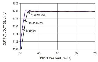
Figure 7. Typical Output Voltage Regulation vs. Input Voltage.
