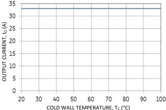
Figure 24. Output Current Derating for the Base Plate QBVW033A0B-H at 48V in in a Cold wall application; Local Internal Air Temperature near module= $80^{\circ}$ C;  $V_{OUT}$  setting anywhere from 6.0V to 12.0V.
