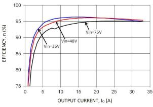
Figure 2. Typical Converter Efficiency vs. Output Current.
