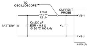
Note: Measure input reflected-ripple current with a simulated source inductance (LTEST) of 12  $\mu$ H. Capacitor CS offsets possible battery impedance. Measure current as shown above.
