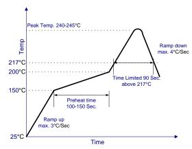
Figure 24. Recommended linear reflow profile using Sn/Ag/Cu solder.
