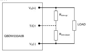
Figure 16. Circuit Configuration to Trim Output Voltage.
