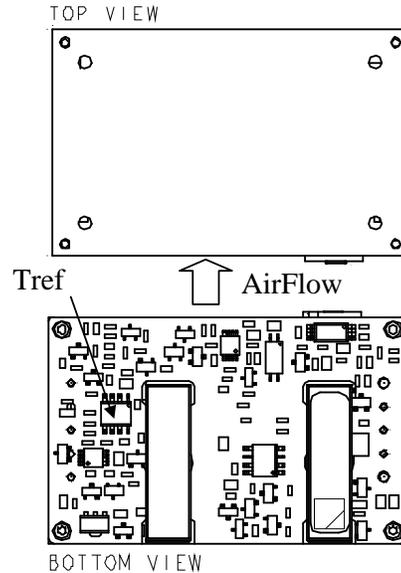
Figure 1.  $T_{ref}$  Temperature Measurement Location
