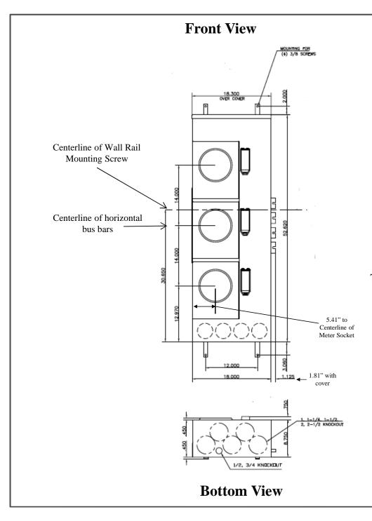
This unit includes factory installed 5th jaw kit (5 terminal unit)
