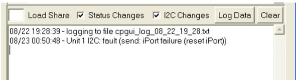
**Load share** – an entry in this table compares the difference in current readings between the modules. If the difference is greater than the value entered, this data will be recorded.
