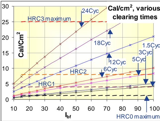
**Fig. 1** Incident energy for a 480V, solidly grounded systems with a 32mm arcing gap and 24" working distance.
