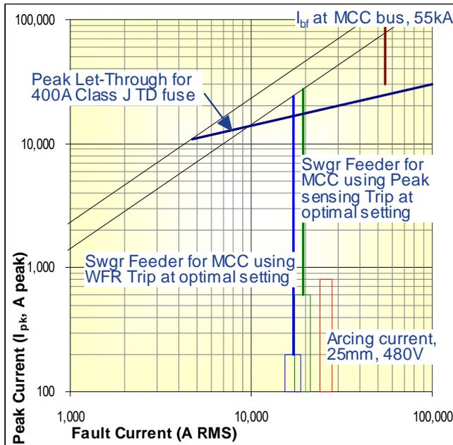
**Fig. 8** Peak and WFR settings above a 400A Class J Time Delay fuse with 55kA available, showing arcing current for 25mm gap at 55kA  $I_{bf}$
