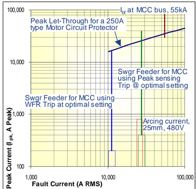
**Fig. 7** Peak & WFR settings above a 250A MCP with 55kA available, showing arcing current for 25mm gap at 55kA  $I_{bf}$
