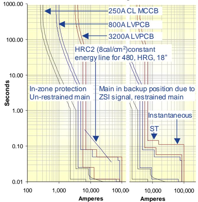
**Fig. 9** Three circuit breakers (250A MCCB, 800A LVPCB & 3200A LVPCB) set selectively up to 65kA & 85kA & with Instantaneous clearing for low in-zone fault currents. Rightmost TCC shows effect of ZSI shift on main CB
