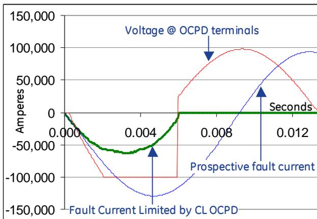
Fig. 3 Modeled peak let-through waveform for a single pole of a CL circuit breaker operating in its current-limiting range.
